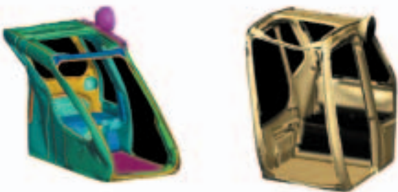
Simulated crash deformation test
