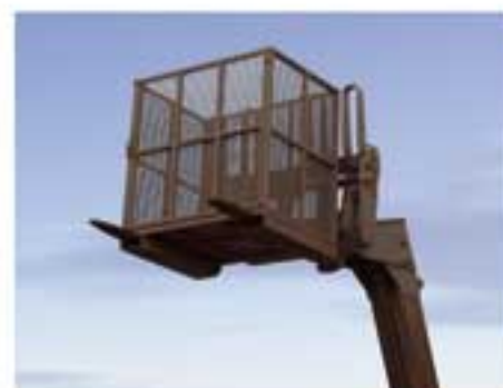
Cestello portamattoni Brick-holder bucket
