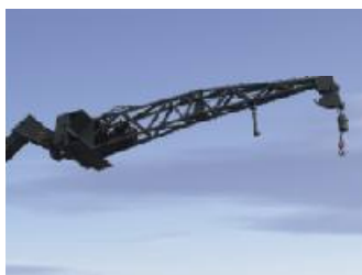
Falcone con verricello idraulico Jib with hydraulic winch
